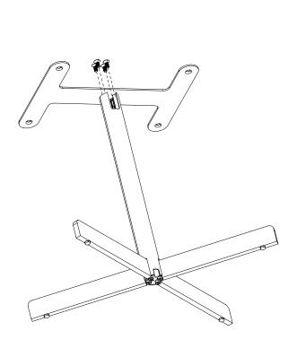
5. Fix the top plate (B) to the tube (E) with the 4 screws (C)
