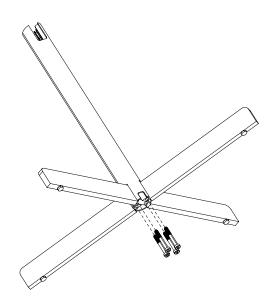
4. Join legs and tube with 4 screws (L)
