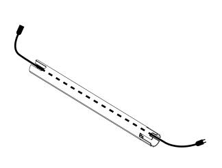
3. insert the power cable through the tube (E)
